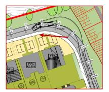
The visibility to private accesses is limited in locations due to the proposed horizontal alignment and a strip of vegetation which is used to separate properties. Insufficient visibility to vehicles reversing out of private driveways may lead to possible side-on collisions, as drivers exit their property and enter the carriageway.
